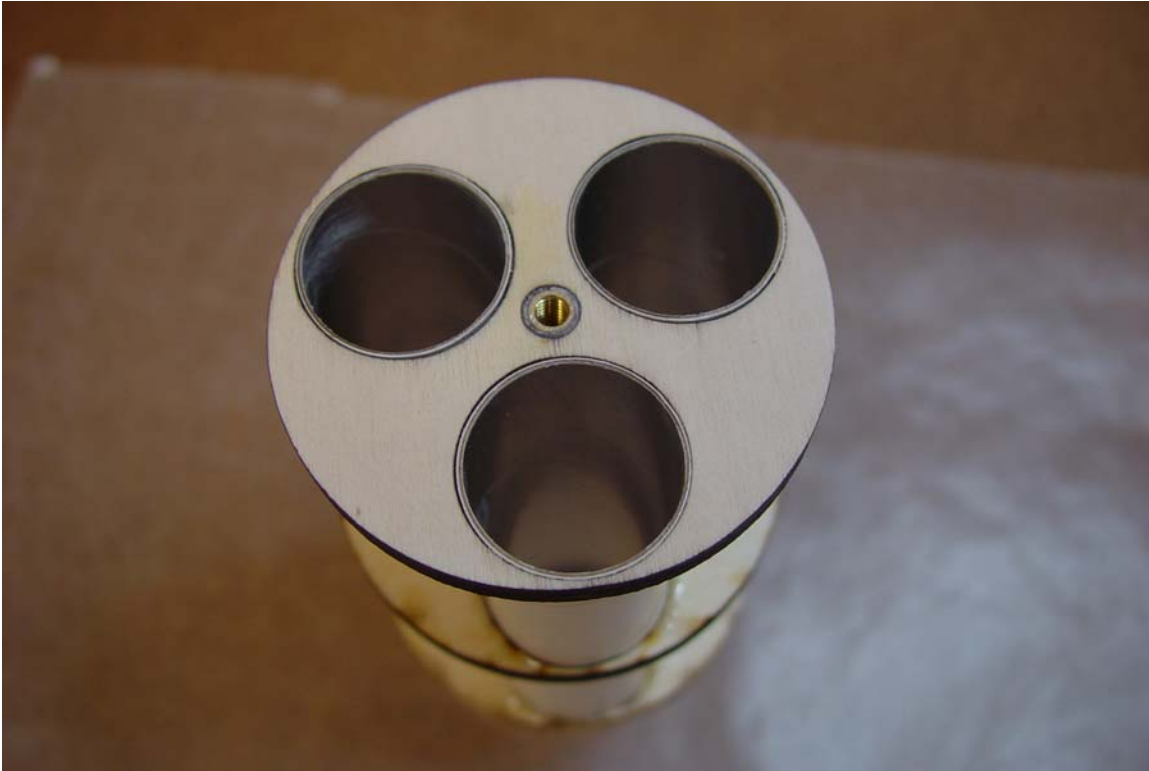
Photo 5: Aft Centering Ring in Place
