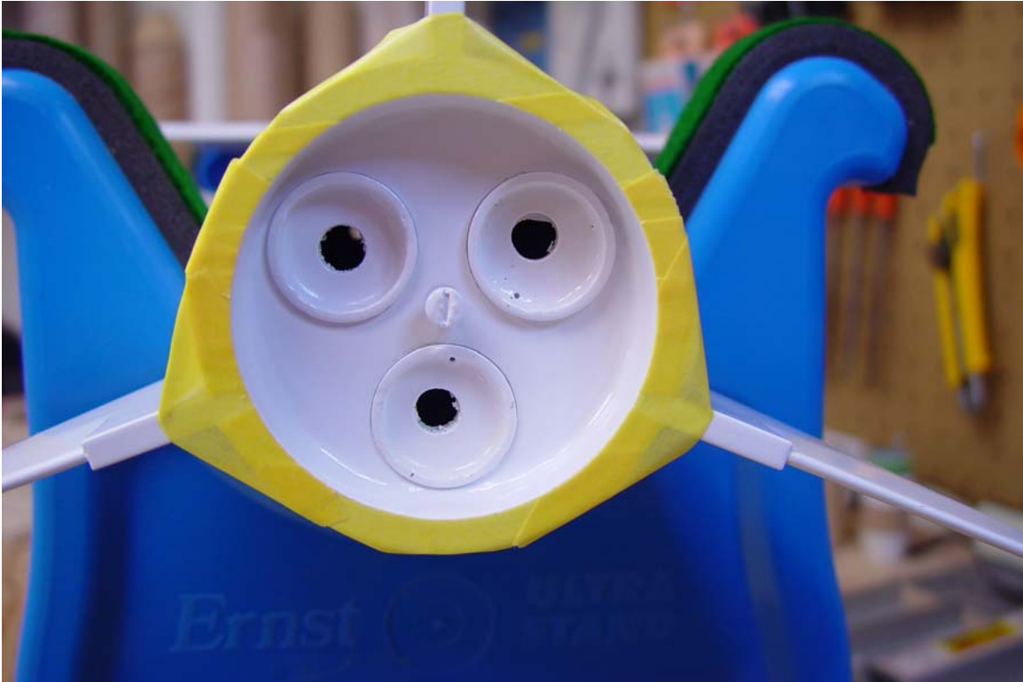
Photo 2: Interior Mask Removed; Engine Mounts Plugged
