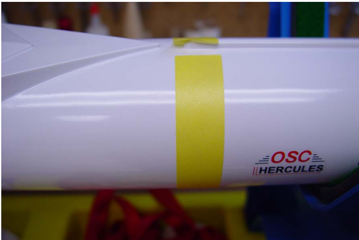
Photo 12: Masking Tape Guide in Place
