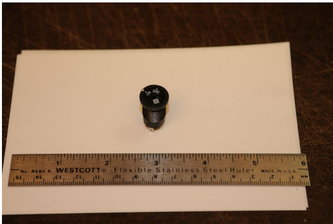
Photo 3: Altimeter Power Switch
