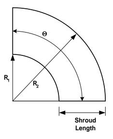
Figure 3: The Transition Shroud in Plan Form.
